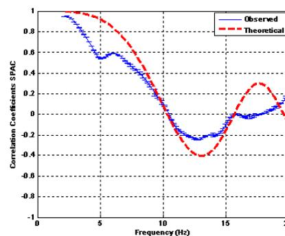
Fig. 2 Autocorrelation coefficients averaged observed and their fit to zero order Bessel function.
