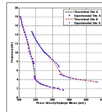
Fig. 4 Experimental (dots), and theoretical (dashed line) Phase velocity dispersion curves
