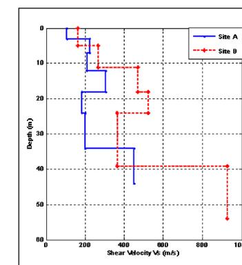
Fig. 5 Obtained shear wave velocity model profiles for sites A and B.
