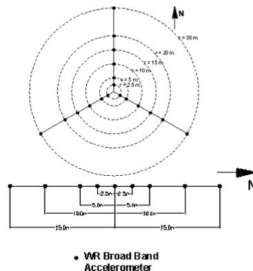
Fig. 1 Top: Geometry of the radial stations, bottom Geometry of the linear stations for ambient vibration detection
